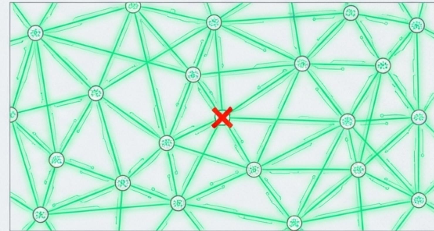
A mesh network map. One node has a red "X", but all surrounding nodes remain connected and lit via triangular mesh lines.
